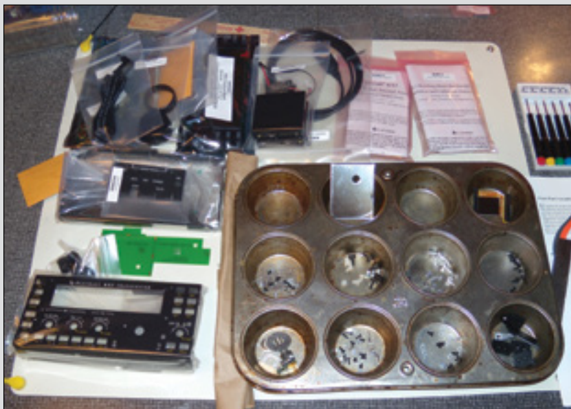
Figure A — The KX3's parts are sorted into the cups of a muffin pan for easy identification as called out in the instructions.
