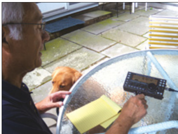
Figure 1 — The KX3's small size makes it a natural for camping or picnic table use. Here the author uses the KX3 in "minimalist" mode, using the internal battery and speaker with the optional paddles attached. Just the connection of an antenna has him on the air.
