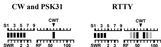
In RTTY or *radioteletype* modes (FSK D, AFSK A; pg. 18) mark and space tones are represented by three bars on either side of the CWT pointer. If no RTTY signal is present, you’ll see the “ghosting” effect shown above. As you tune in an RTTY signal, the number of solid bars will increase. Keep tuning until you see a rough balance between left and right solid bars during an RTTY transmission.
