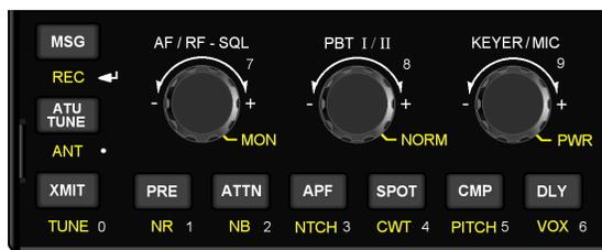
First, tap **FREQ ENT**. Then enter up to three MHz digits, optionally followed by a decimal point (**ATU TUNE** switch) and up to three kHz digits. Next tap **←** (**MSG** switch) to accept, or any other switch to cancel. **Examples:**
