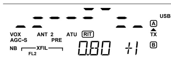
The center frequencies of the 8 audio EQ bands are 50, 100, 200, 400, 800, 1600, 2400, and 3200 Hz. To select a band to change, tap **[1-8]** on the keypad. For example, tapping **[1]** selects the 50-Hz band.
