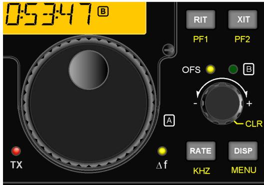
**VFO A** normally controls both the receive and transmit frequency. Most contacts occur between stations tuned to about the same frequency, so if you use VFO A to tune in a signal clearly, there's a good chance they'll hear you when you transmit.
