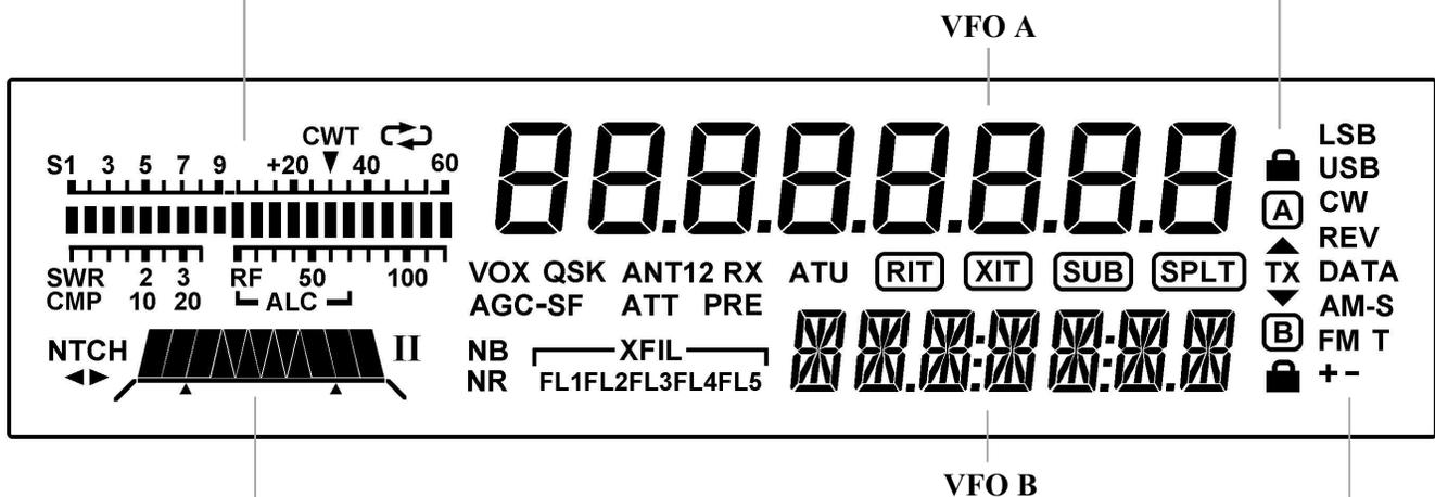
**Filter Passband Graphic:** Shows location of receive filter passband (pg. 12)
