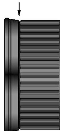
Use the supplied 5/64" (2 mm) Allen wrench to loosen the set screw.
